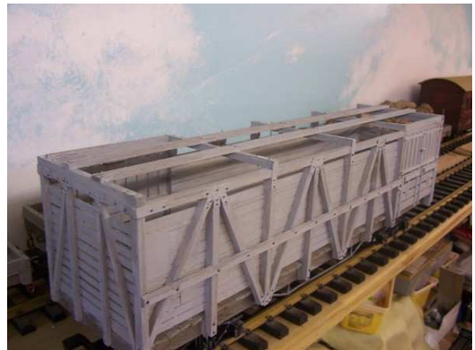
The base relief that the pin heads 'show' accentuates the bolt, nuts and washers.
