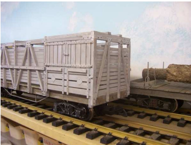
The base relief that the pin heads 'show' accentuates the bolt, nuts and washers.
